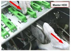
2. Release the three latches marked to separate the front bezel from the housing case, then lead the cables out.
